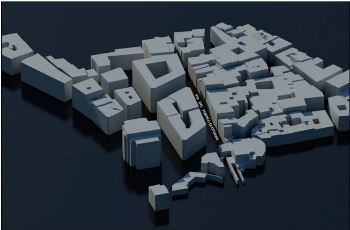
Fig. 2: 3d representation of Jewish Ghetto area. Realistic simulation of solar irradiation on the building curtain on “Portico di Ottavia” street. (on the right side). Time: 21 June 5:00 pm. Facades are still strongly exposed. Sun exposure continues for all day long.
