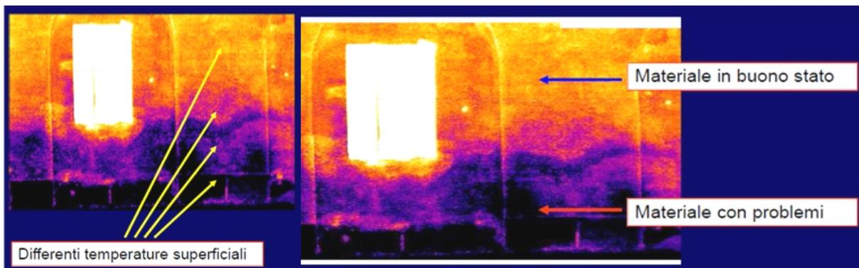
Fig. 11: Thermographic mapping
